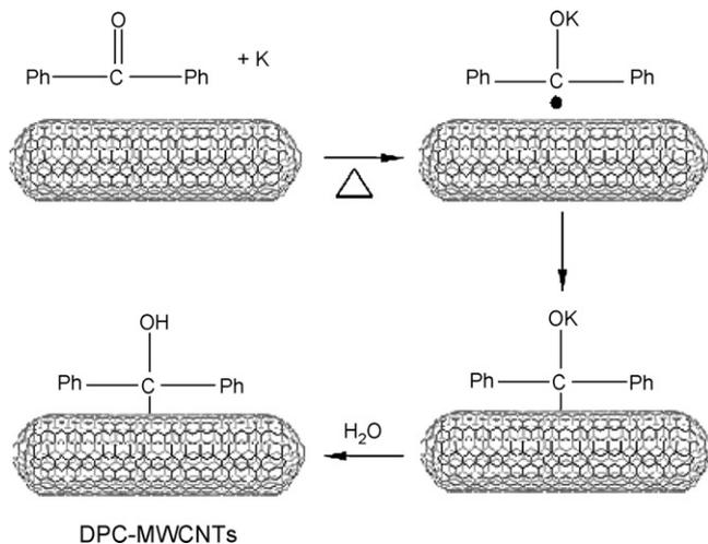
**Fig. 2.** Chemical reaction for the preparation of DPC-MWCNTs [15].
