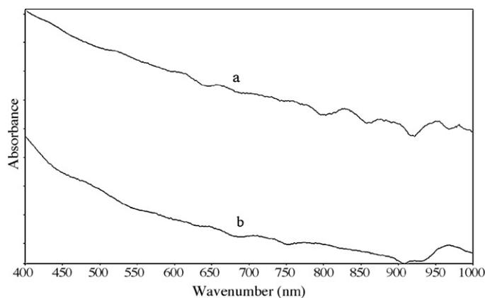
**Fig. 4.** UV-vis absorption spectroscopy in dimethylformamide: (a) Pristine MWCNTs and (b) DPC-MWCNTs.
