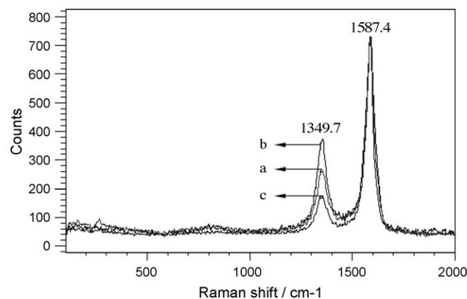
**Fig. 3.** Raman spectra of: (a) Pristine MWCNTs, (b) DPC-MWCNTs and (c) DPC-MWCNTs after TGA.
