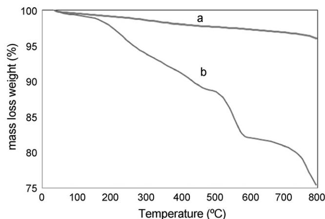
**Fig. 5.** TGA result for (a) Pristine MWCNTs and (b) DPC-MWCNTs.
