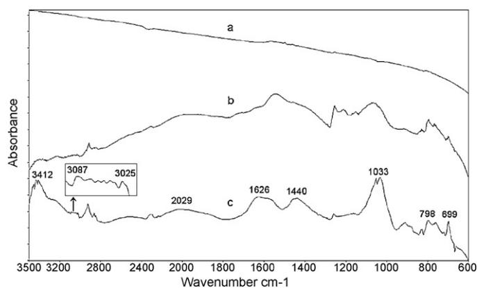
**Fig. 1.** FTIR spectra of (a) Pristine MWCNTs, (b) DPC-MWCNTs (5 days) and (c) DPC-MWCNTs (10 days).
