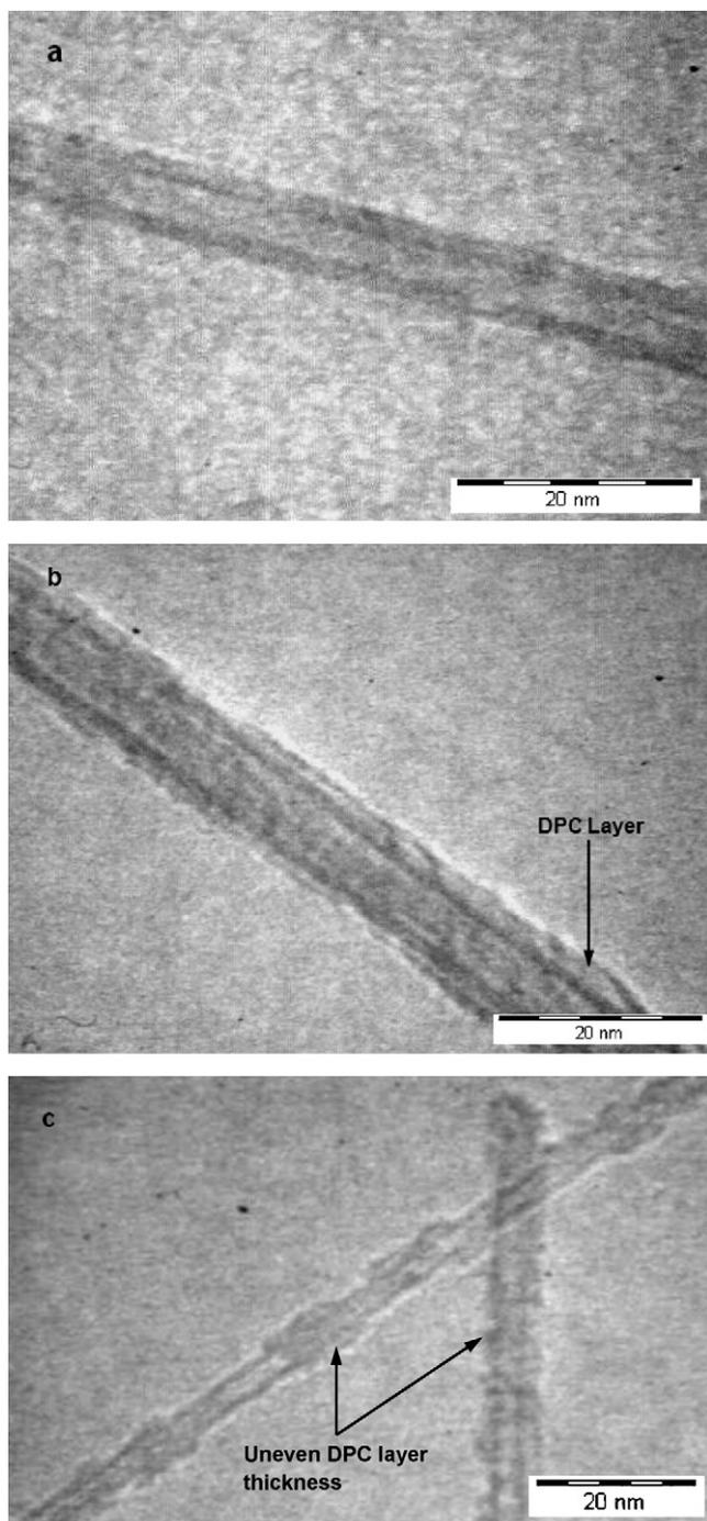
**Fig. 6.** TEM image of (a) Pristine MWCNT (at  $\times 100k$  magnification), (b) DPC-MWCNT (at  $\times 100k$  magnification) and (c) DPC-MWCNT (at  $\times 60k$  magnification).
